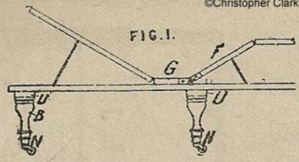
Invalid and other couches.—The adjustable framing is formed in hinged sections, the hinges connecting the parts G, F being each secured to the body of the sofa by a 1-shaped bar connected to or in one with the hinge-pins. For removable legs, a rod carrying the castor N passes through the leg and screws into a nut fixed in a block U. For spring bottoms, spiral wire springs are secured by fixings or clasps to the framework, and are connected at the crossings by clasps or loops.
